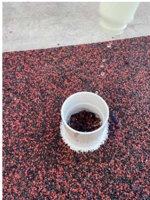
Water seeping through sample material
